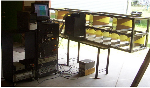
Fig. 8. The real-time S-band radar imaging system.
